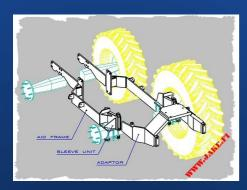
JAKE Mounting Kit for mounting a forestry crane, digger or even a loading crane or a machine arm mulcher on a tractor
