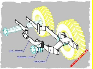
under the sleeves. Turn the boom backward, telescope fully out, lift the grapple ca. 3 metres from the ground, lower down the main boom with some speed and stop the move quickly. This forces the adaptor to come loose. N.B ! Only loose the upper locking bolts 10 mm, do not remove them yet ! This prevents the adaptor from coming completely out of the sleeves accidentally !
