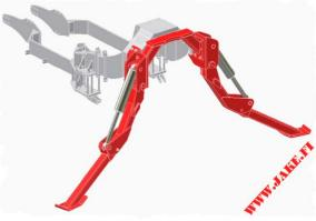
the JAKE Heavy Duty Legs are not wider than the tractor. The maximum width of the legs at the ground position is approximately 5,0 metres.
