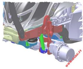
for the axle with only oscillation and JAKE SPN Front Axle Stabilizer for the axle with both oscillation and suspension. Both models have own versions for a front loader tractor and for a front linkage tractor.
