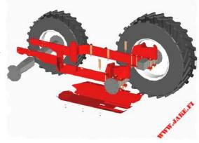
**Armours** are mainly fastened to the Aid Frame of the **JAKE Mounting Kit**. If a tractor is not equipped with the **JAKE Mounting Kit**, the Aid Frame must be ordered together with the **JAKE Armour**.
