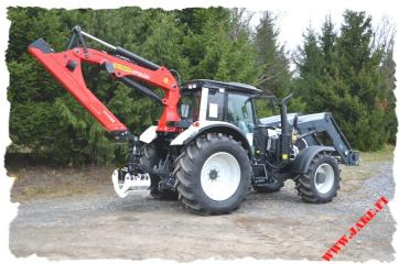
The **JAKE 904** makes using the crane versatile as the crane mounted on the tractor can be combined with other devices connected to a 3-point linkage and a trailer hitch usually with no limits (except for parallel cranes).
