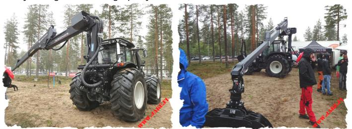
The **JAKE 900** makes using the crane versatile as the crane mounted on the tractor can be combined with other devices connected to a 3-point linkage and a trailer hitch usually with no limits (except for parallel cranes).
