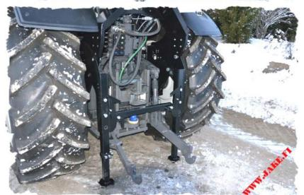
4. Lift the lower linkage arms that much that the locking hooks turn under the arms. Do not lift more yet.
