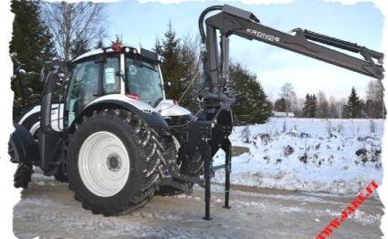
ALWAYS BE SURE THE TRACTOR STAYS STILL AND THAT THE CRANE CAN NOT TIP OVER WHILE WORKING BETWEEN THE TRACTOR AND THE CRANE!
