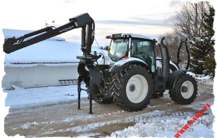
**N.B!** The parking legs do not stand backwards or forward moving of the crane!
